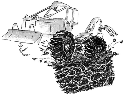
Soil compaction after 1 pass
