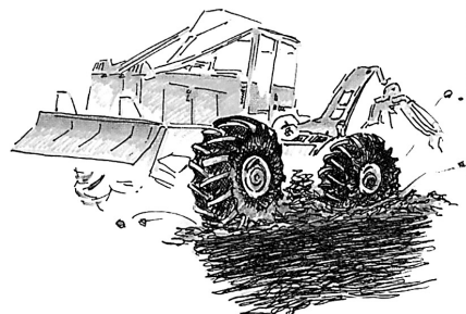
Soil compaction after 12 passes
